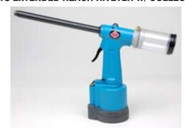
This specialty riveter is for reaching into those really deep areas. Vacuum collection system keeps stems safely stowed in collector.
